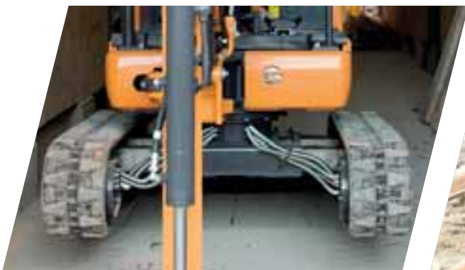
Extended tracks to increase stability while working
