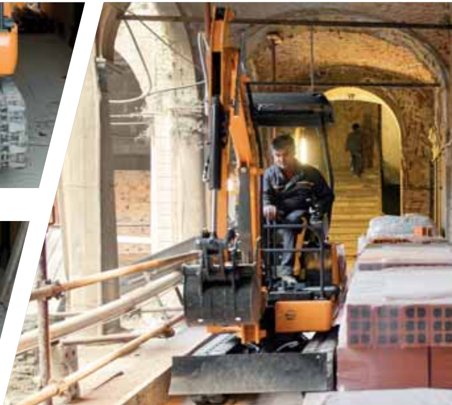
Retracted tracks to access confined spaces
