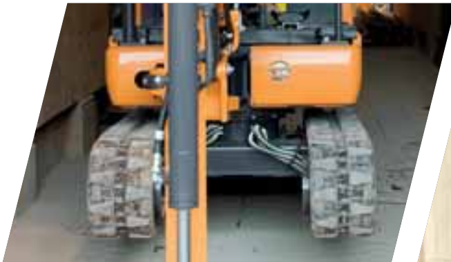
Retracted tracks to access confined spaces
