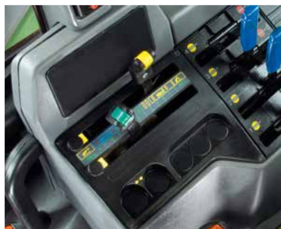
Two levers are used to control the rear lift links: the yellow lever raises or lowers the implement; the green lever is used to select the type of control (position, draft and mix). The blue levers operate the various auxiliary spool valves — single acting, double acting, kickout or detent.
