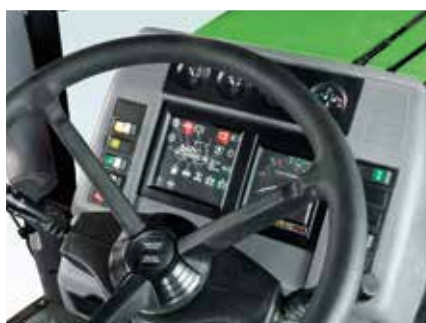
The Agrotac instrument panel: clear and complete information on the operating status of the tractor.
