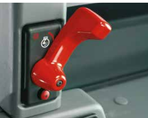
Engine speed controlled by a lever on the cab door post, with the facility of memorizing a set speed.
