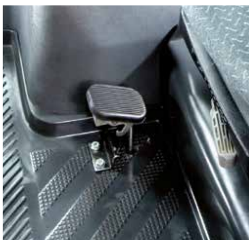
Front and rear differentials with 100% locking action are conveniently pedal operated. (Agrotac 610-620).
