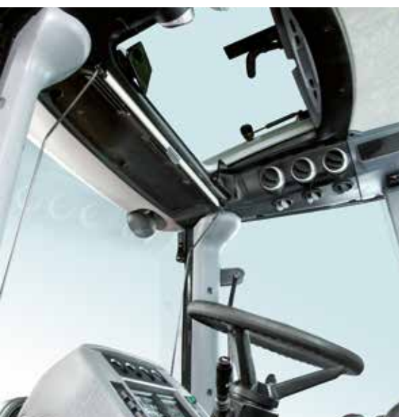
An uninterrupted view topside. The high visibility cab features a glass hatch that takes up almost the entire roof area, allowing the driver to keep a constant visual check on operations overhead when using a front loader.
