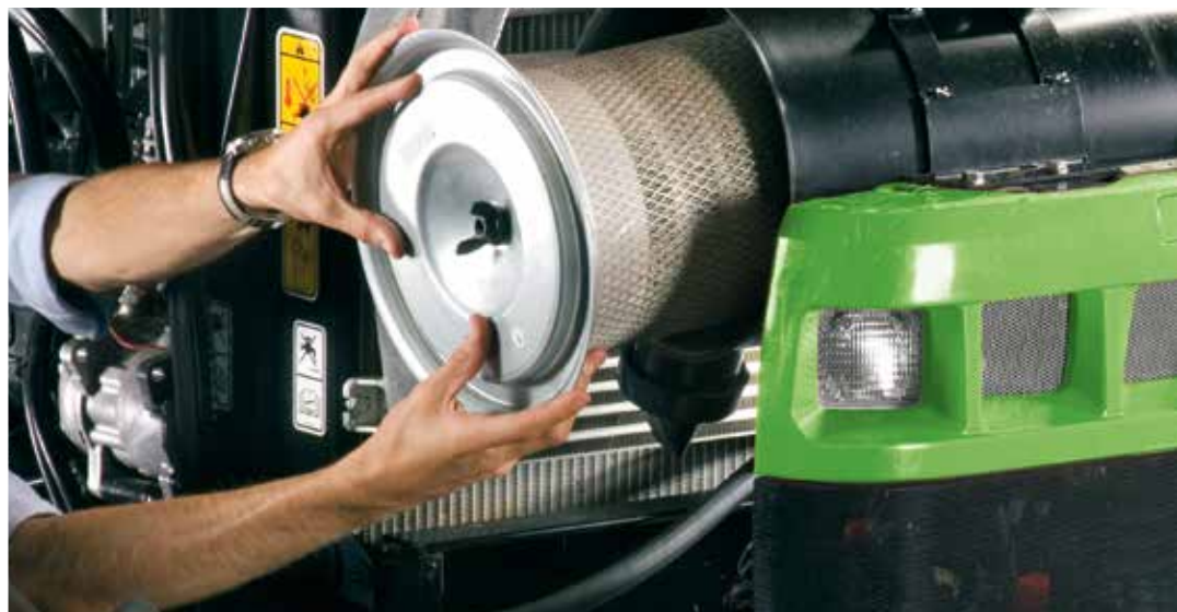
The engine air cleaner is serviced easily and in minutes.
