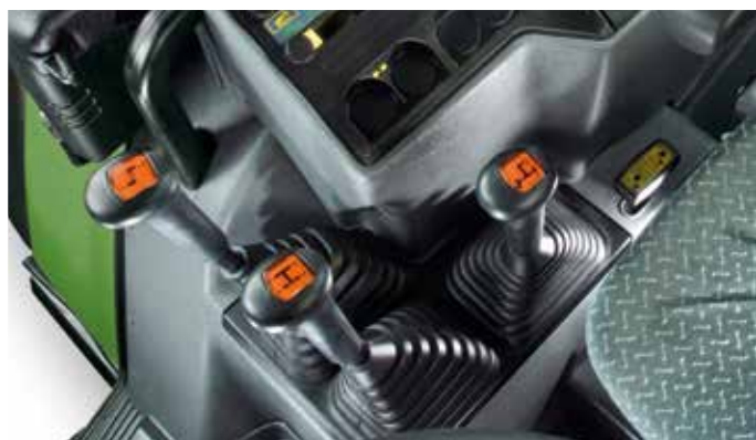
16FWD+12REV transmission with creeper range or 24FWD+12REV with Hi-Lo.
