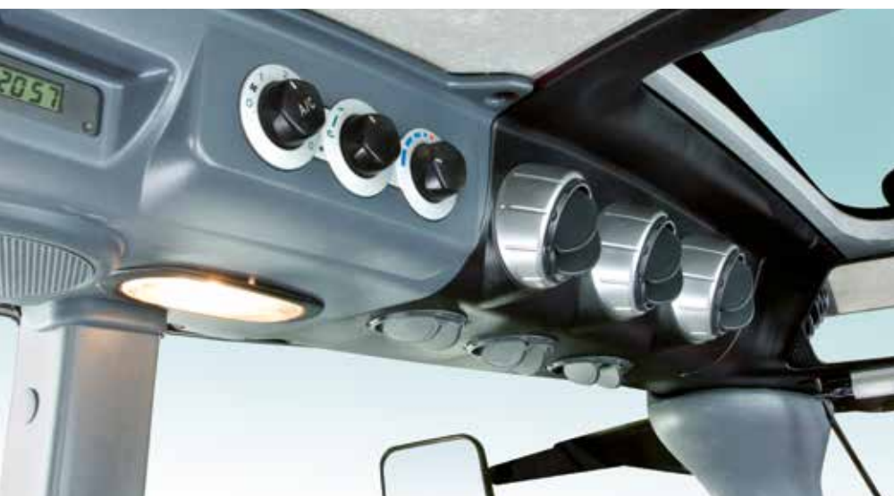
An efficient 4-speed ventilation system circulates a perfectly measured flow of air through 18 adjustable vents, regulating the temperature inside the cab at a level guaranteed to provide maximum operator comfort, whatever the climatic conditions.
