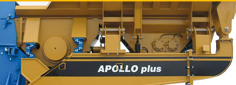
Vibrating feeder with pre-screening, for perfect extraction of fine materials, fitted with brand named ROSTA elements.
