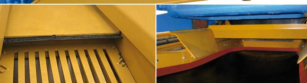
Interchangeable grid with punch plate.
