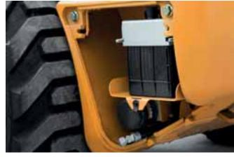
Smart battery and drain hoses access
